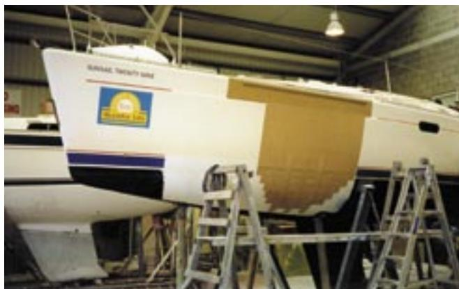
**3** With the insides of the cut-marks tapered, sheets of Melamine hardboard are now used to recreate the hull shape. This is fairly quick, but will it be quite labour-intensive when it comes to flattening back the gel coat that has been laid up against it from the inside.
