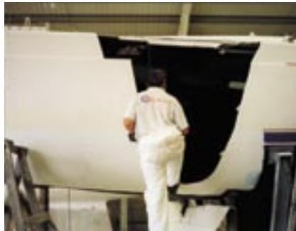
**2** The first job is to cut away all the damage to beyond the last of the stress cracks. A fine snot is used to trace where the hairline cracks finally end. Note how all the antifouling has been stripped for some distance each side of the damage. To get to the hull, much of the internal furniture in this section had to be disassembled.
