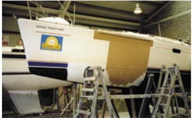
**3** With the insides of the cut-marks tapered, sheets of Melamine hardboard are now used to recreate the hull shape. This is fairly quick, but will it be quite labour-intensive when it comes to flattening back the gel coat that has been laid up against it from the inside.
