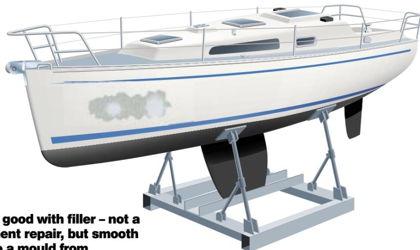
Damage made good with filler – not a strong permanent repair, but smooth enough to take a mould from
