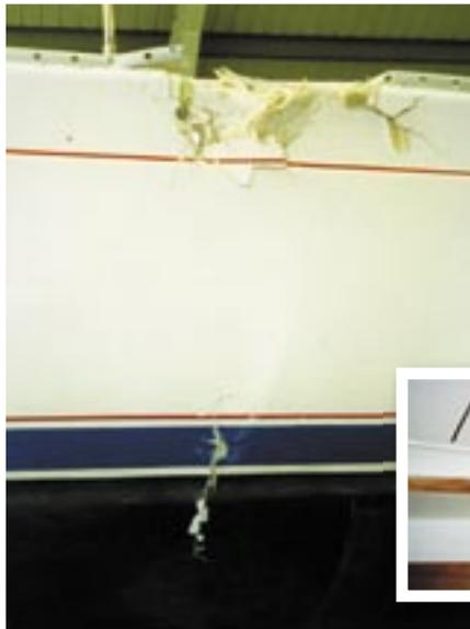
**1** When this Jeanneau was struck by another yacht during a race, the damage seemed relatively light. However, once craned ashore, it was found that the hull had stress cracks from the toerail right down to below the waterline. Inside, the main saloon bulkhead had been shattered.
