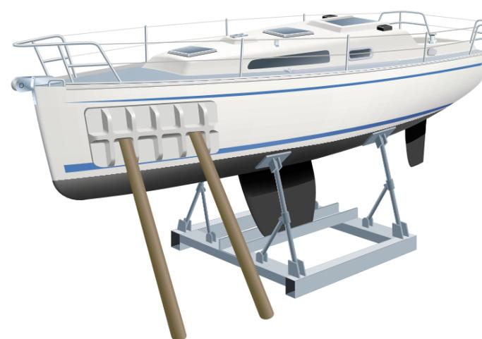
Take a mould from the 'made good area'. Then chop out the damage and rebuild from the mould as in steps 4 and 5 (above)
