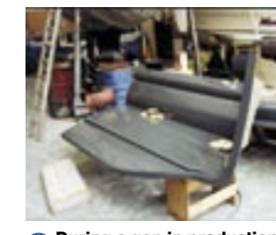
**2** During a gap in production the Windy factory was able to supply a cast from the mould, from which this female mould was made.
